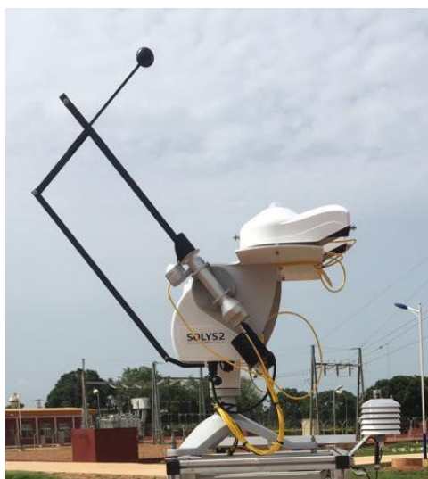
Figure 22 : Tracker installé / Installed tracker
