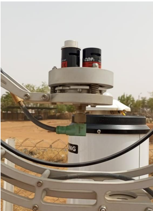
Figure 71: RSI installé, mis à niveau et connecté / RSI sensor head installed, levelled and connected.
