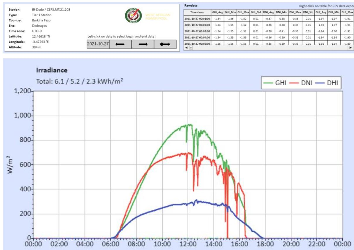
Figure 42 : Irradiance measurement. GHI, DNI and DHI.
