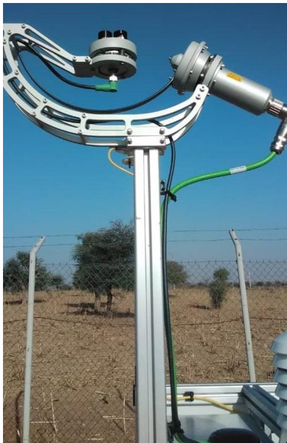
Figure 55: RSI installé / Installed RSI.
