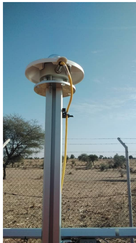
Figure 52: Pyranomètre CMP10 installé (GHI) / Installed CMP10 pyranometer (GHI).
