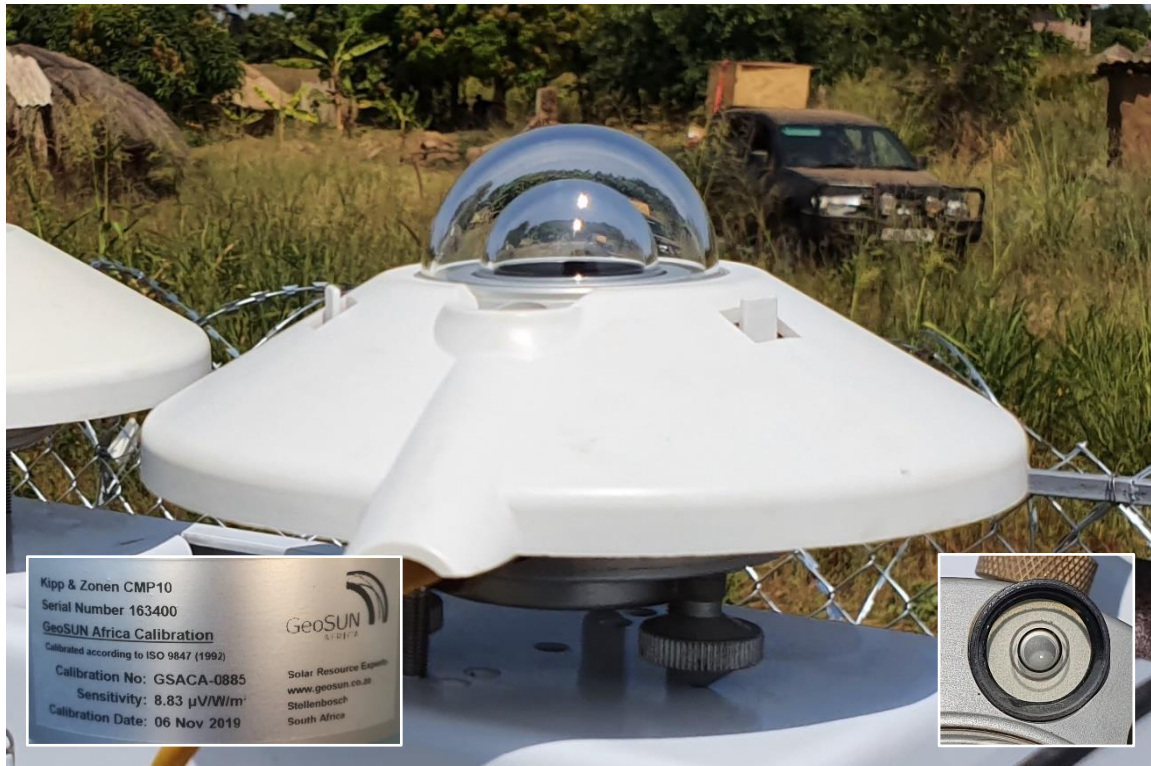
Figure 7: GHI (1) Pyranometer Installation
