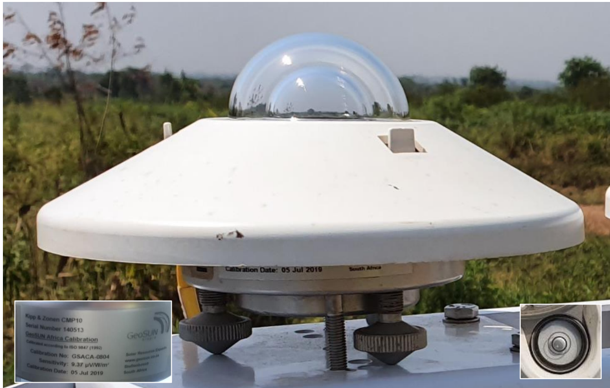
Figure 7: GHI (1) Pyranometer Installation
