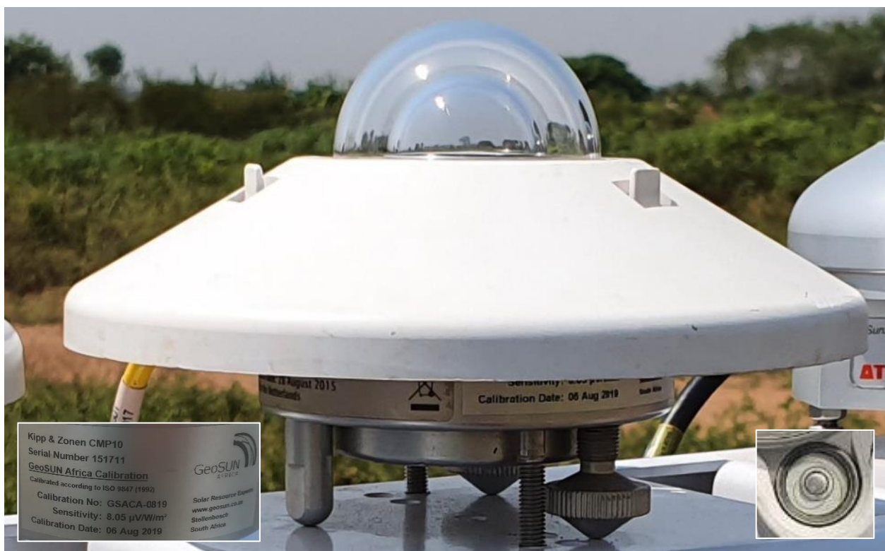
Figure 8: GHI (2) Pyranometer Installation
