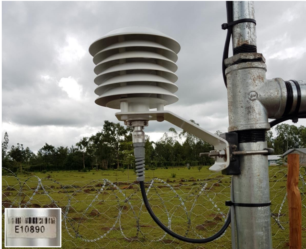
Figure 11: Thermometer and Hygrometer at 2 m
