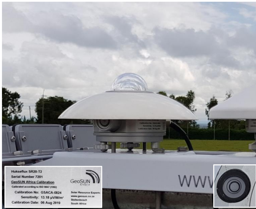
Figure 7: GHI (1) Pyranometer Installation
