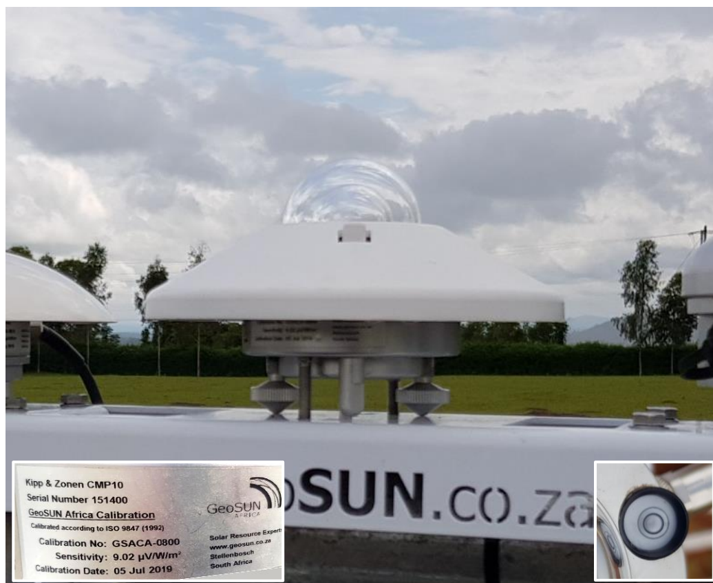
Figure 8: GHI (2) Pyranometer Installation
