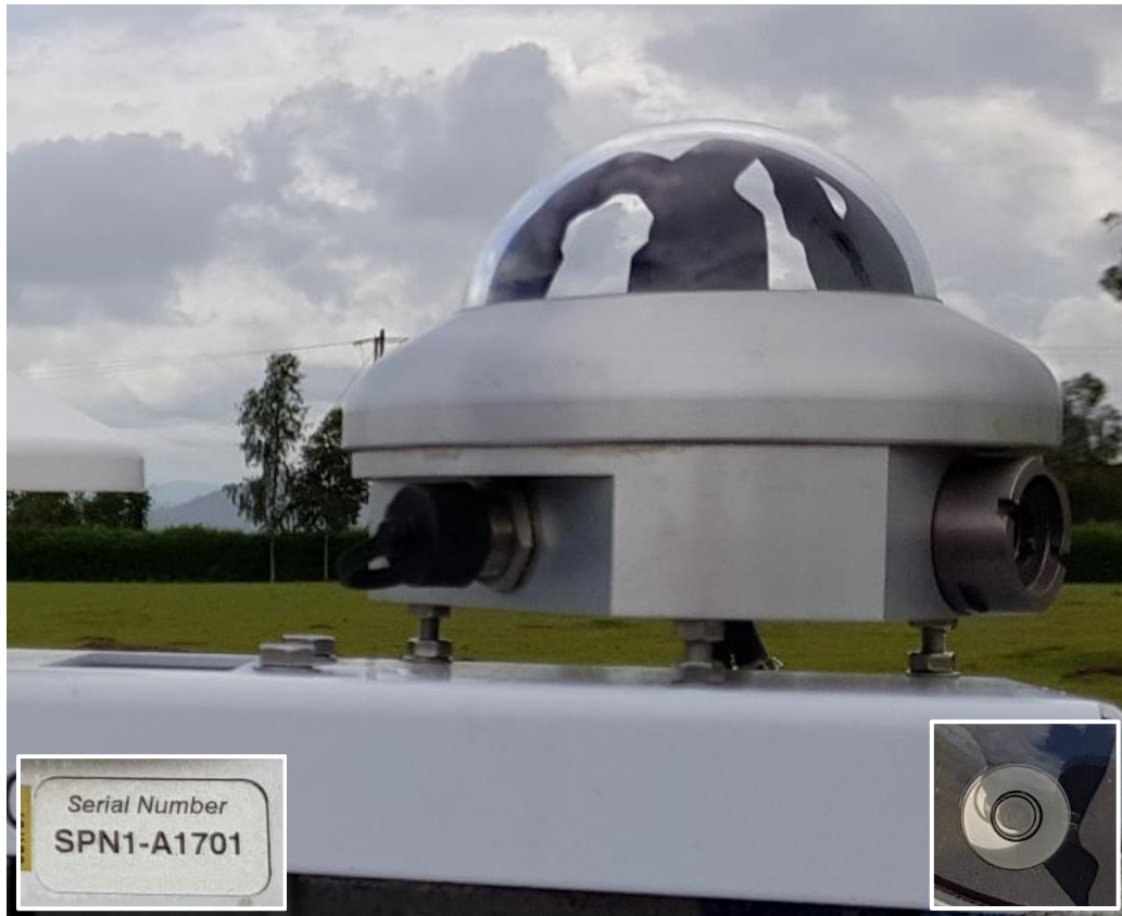
Figure 9: DHI Pyranometer Installation
