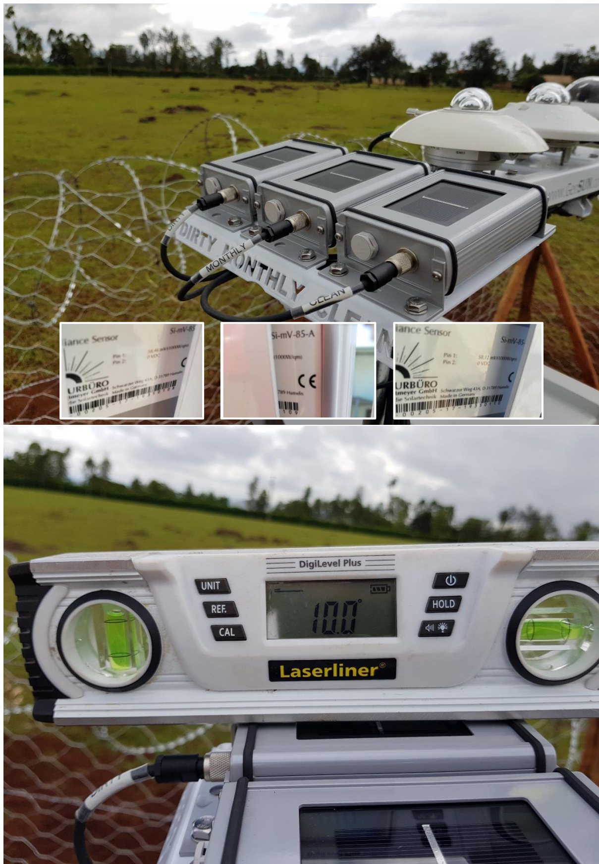
Figure 15: Reference Cells at 10° North
