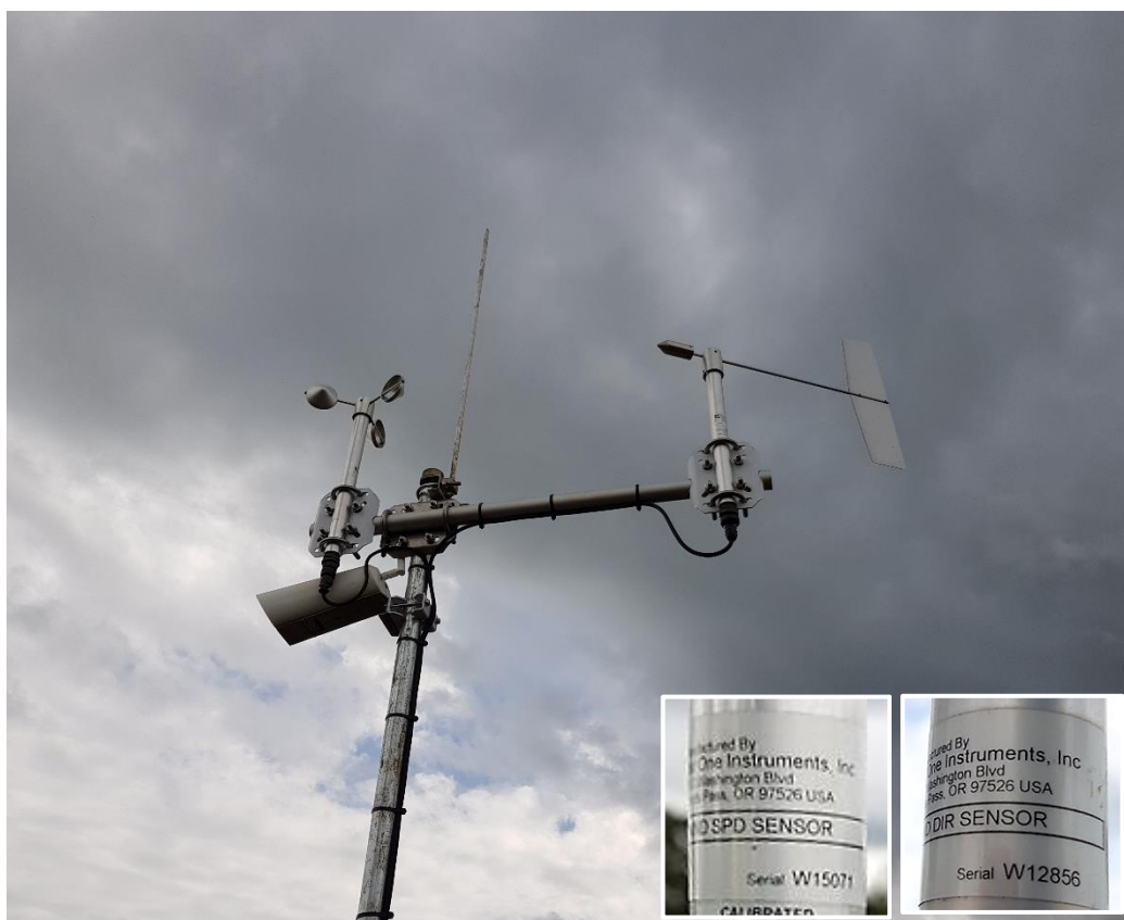
Figure 10: Wind Instruments at 3 m
