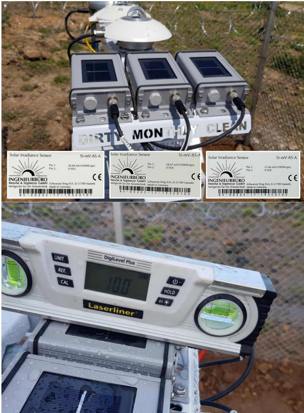
Figure 15: Reference Cells at 10° South
