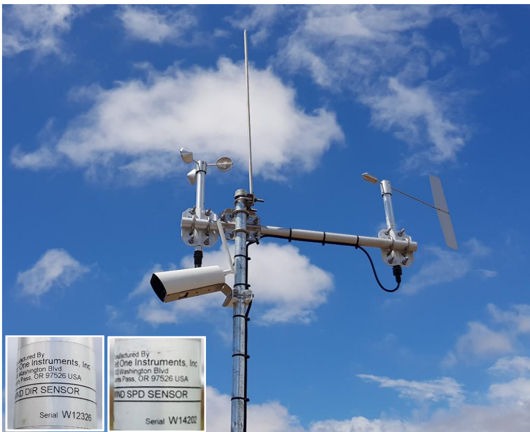
Figure 10: Wind instruments at 3 m
