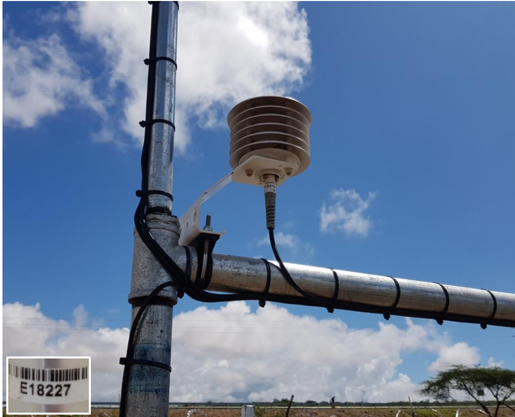
Figure 11: Thermometer and Hygrometer at 2 m
