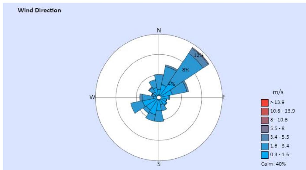
Figure 46 : Wind direction measurement.
