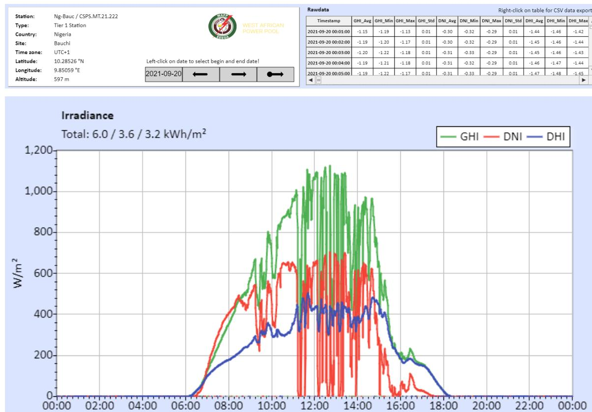
Figure 41 : Irradiance measurement. GHI, DNI and DHI.
