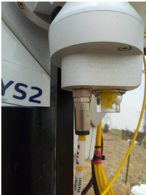
Figure 82 : Changement du dissécant de Pyrheliometer / Change of pyrheliometer desiccant.
