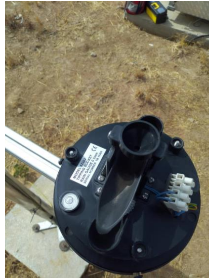
Figure 85: Ruteur LTE / Rain sensor cleaning and levelling.
