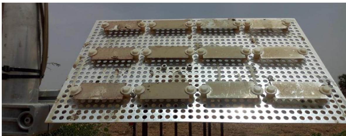
Figure 91: Echantillonneur de corrosion / Corrosion sampler.
