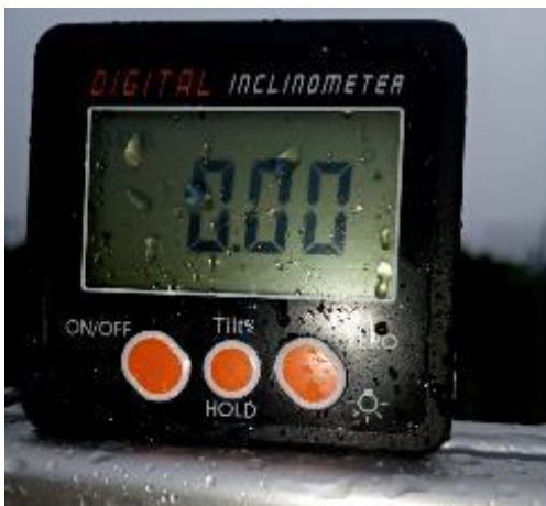
Figure 27 - Rain sensor mounting bar leveling
