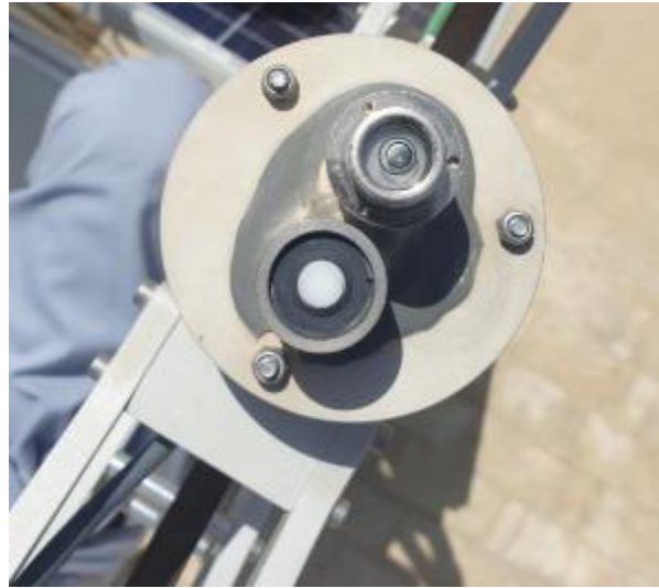
Figure 22 - Sensor levelling of the RSI (2)
