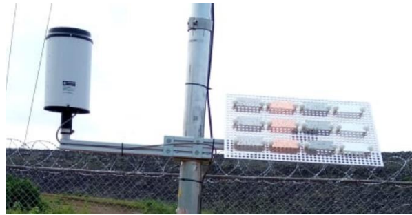
Figure 26 - Rain sensor and corrosion sampler
