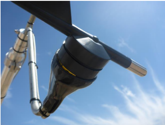
Figure 15 - Wind direction sensor north mark aligned with mounting cantilever and north direction
