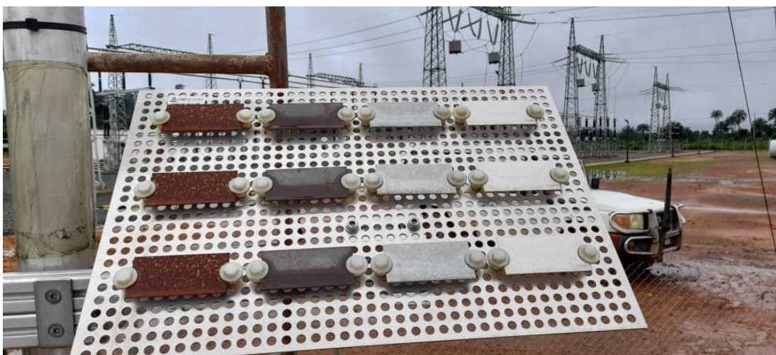
Figure 86: Echantillonneur de corrosion / Corrosion sampler.
