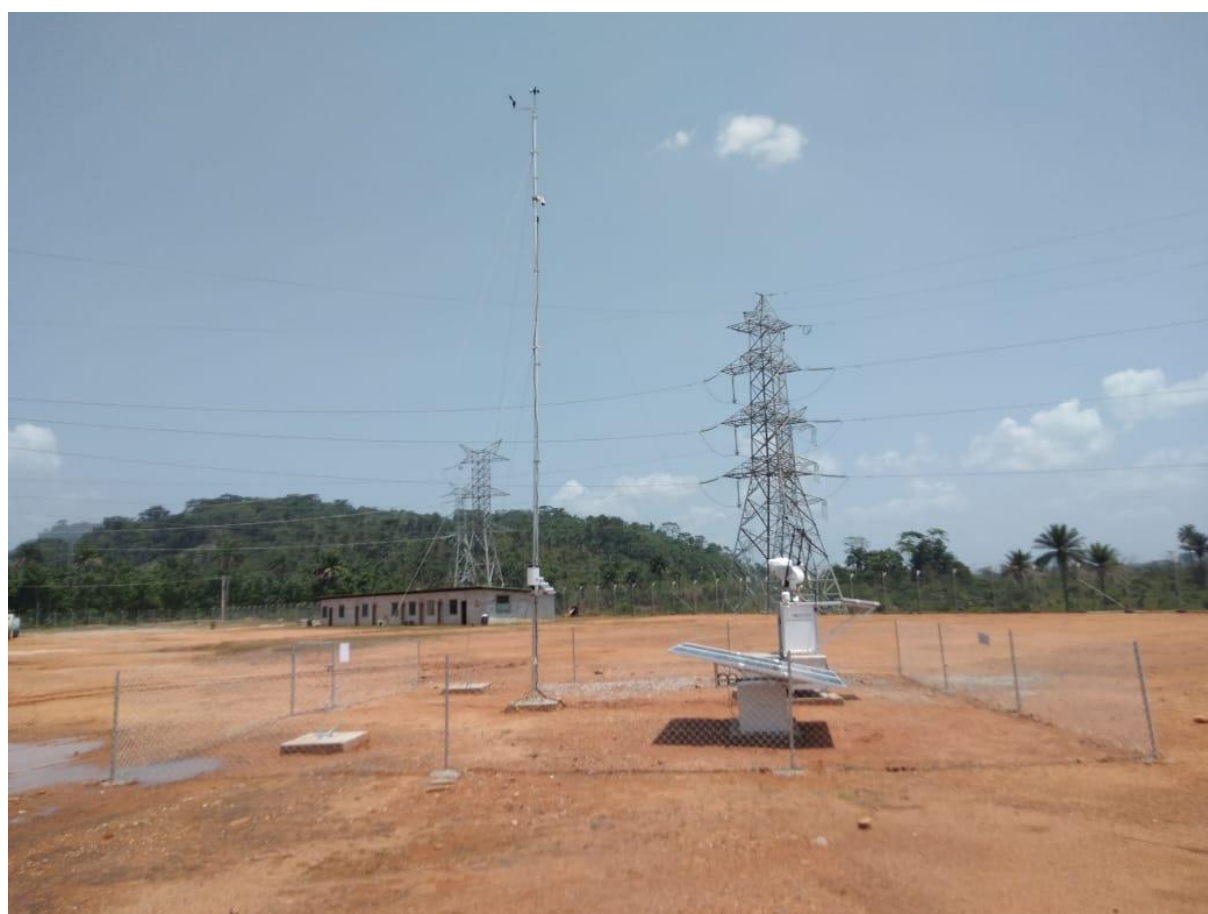
Figure 2: Station météorologique automatique de Yekepa, Liberia / Automatic weather station in Yekepa, Liberia.
