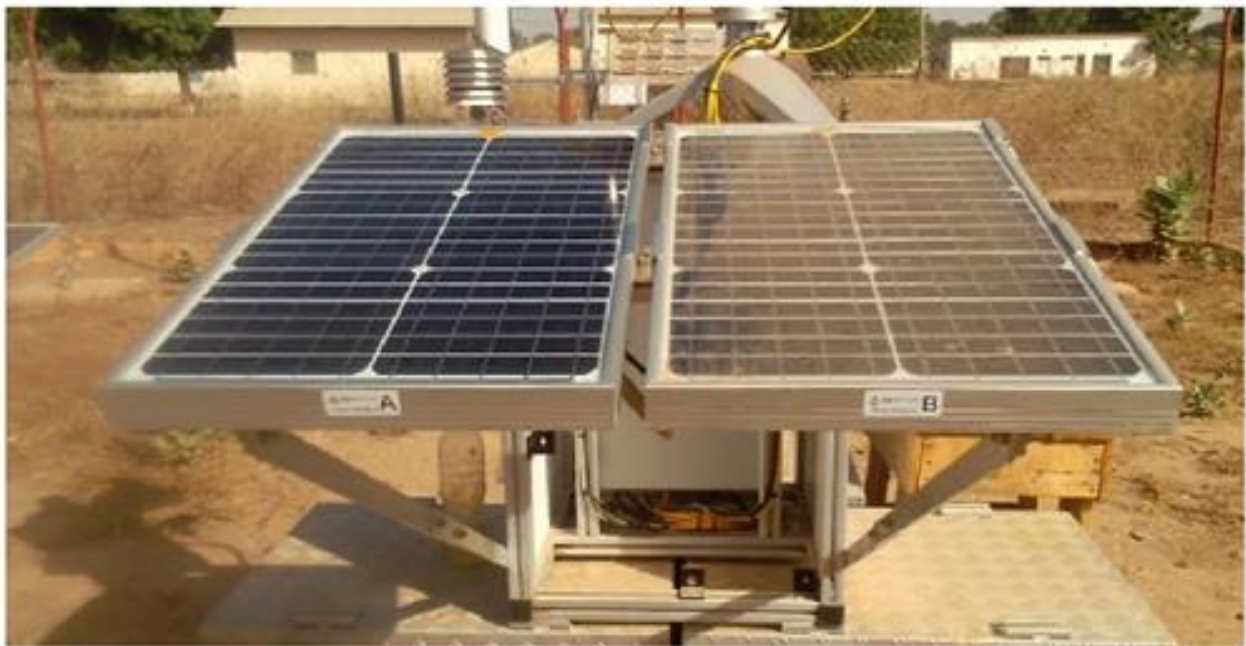
Figure 31: PV-soiling system with the clean reference panel (modA) and the measurement panel (modB). The measurement panel is kept clean by regular cleaning by the local maintenance staff whereas the measurement panel is allowed to accumulate soiling over time
