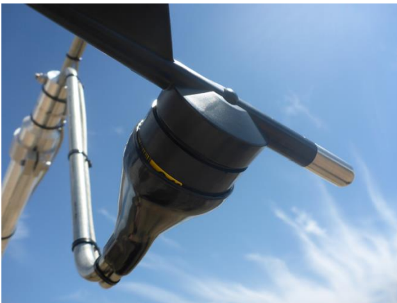
Figure 47 - Wind direction sensor north mark aligned with mounting cantilever and north direction
