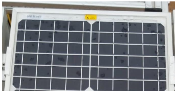
Figure 68 - PV-S system reference panel A (clean panel)
