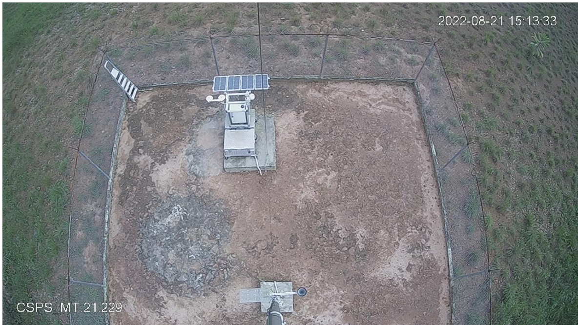
Figure 96: Security camera view (the temporarily installed reference sensor can be seen right next to the permanently installed sensor on top of the weather station)
