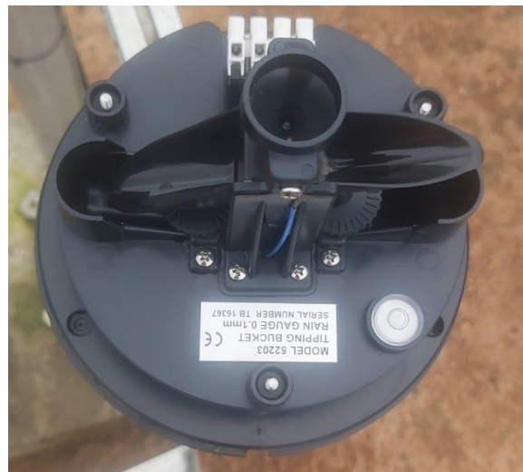
Figure 104: Rain sensor levelling
