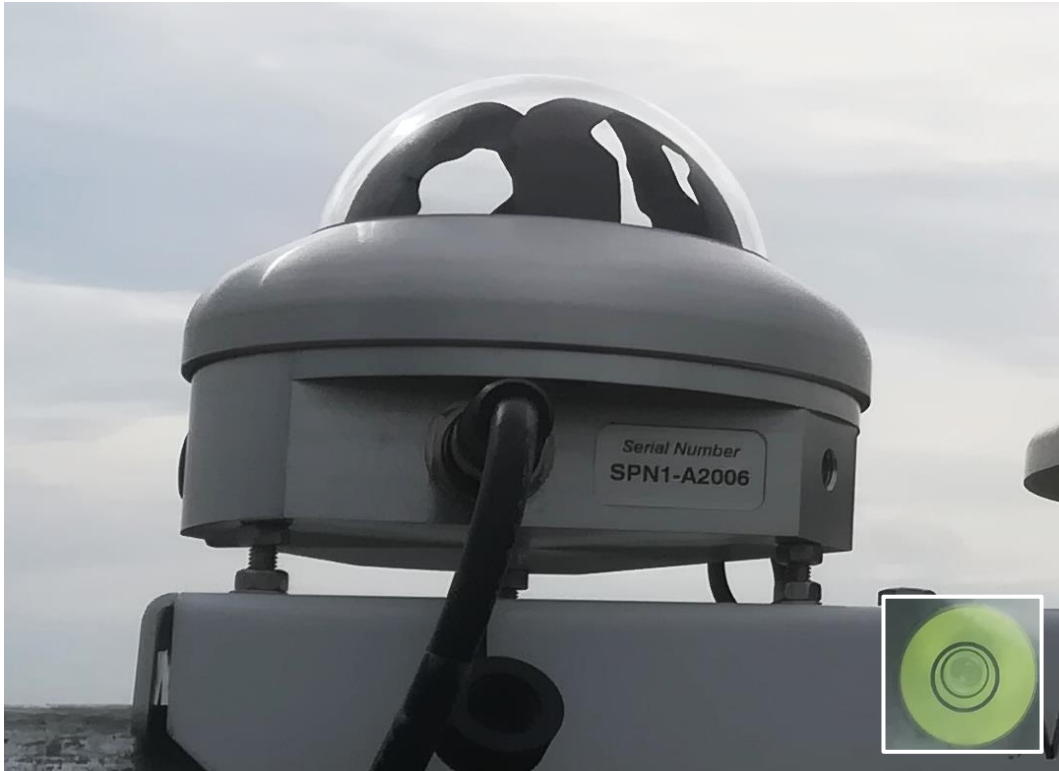
Figure 9: DHI Pyranometer Installation
